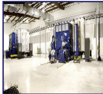
L.A. Darling chose the Nordson Excel 2000 System with Versa-Spray II automatic guns because it required a powder coating system with reclaim capability that could provide the throughput and efficiency needed in a lean environment.
