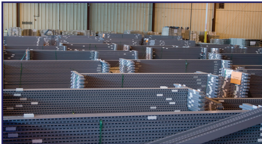
L.A. Darling coats scores of different styles of parts each day, including four-way garment racks, end frames, and shelving decks to wire grid.
