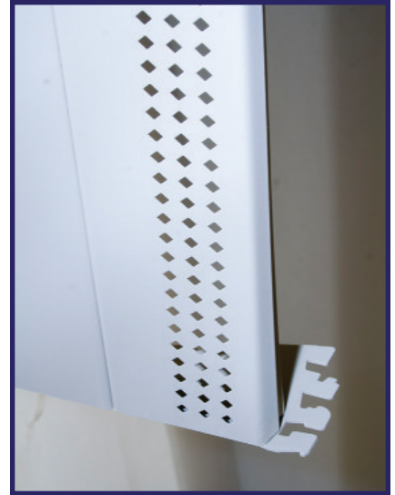
L.A. Darling often powder coats over existing paint on the refurbished fixtures, making accurate control of mil thickness critical.
