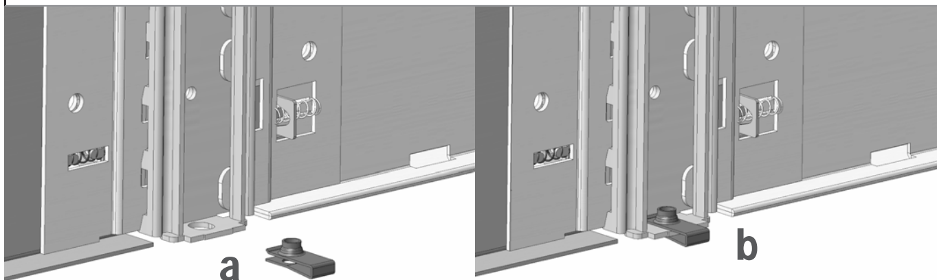
End standards get one (1) clip and center standards get two (2) clips
