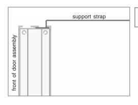
With the front of the door assembly facing away from you (door handles are away from you) slide the support straps into the channel closest to you about 8" from each end.
