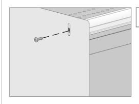
Secure the end panel to the top shelf using one (1) 10-32 x 1/2" machine screw, washer and hex nut per end panel. The washer goes inside the security case with the nut.
