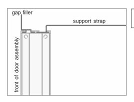
With the front of the door assembly facing you slide the gap filler in from one end to the other so the gap filler is centered in the frame of the door assembly.
