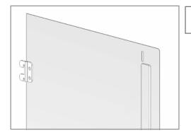
Apply one piece of double face tape to the inside of each end panel (end panel hooks face in). If the height of the end panel is shorter then the length of tape trim the tape to run between the two holes in the end panel. If the end panel is taller then the length of tape cut the tape in half and apply each half one just below the top hole and the other just above the bottom hole as pictured to the left and below.
