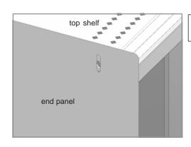
Hook the end panels into the slots on the uprights so the hole in the end panel aligns with the keyed hole on the shelf as pictured to the left. When installed the end panel should overlap the top shelf slightly as well as the bottom shelf or deck.
