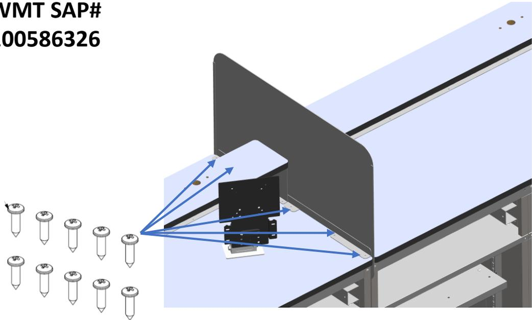
**53519402--- Hardware Kit Consist of: (5ea) #8-10 Course Thread Pan Head Particleboard screws
