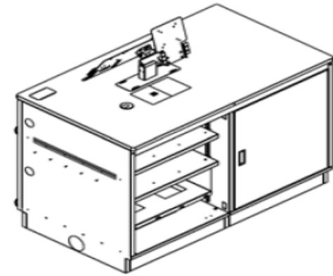
**Step 2: Attach the Bumper End Caps to the cabinet using the pre-punched holes in the cabinet with the Two screws provided.**
