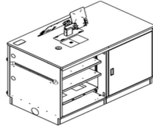
**Step 3: Snap the bumper rail onto the track and continue to the second row of bumper on the cabinet.**
