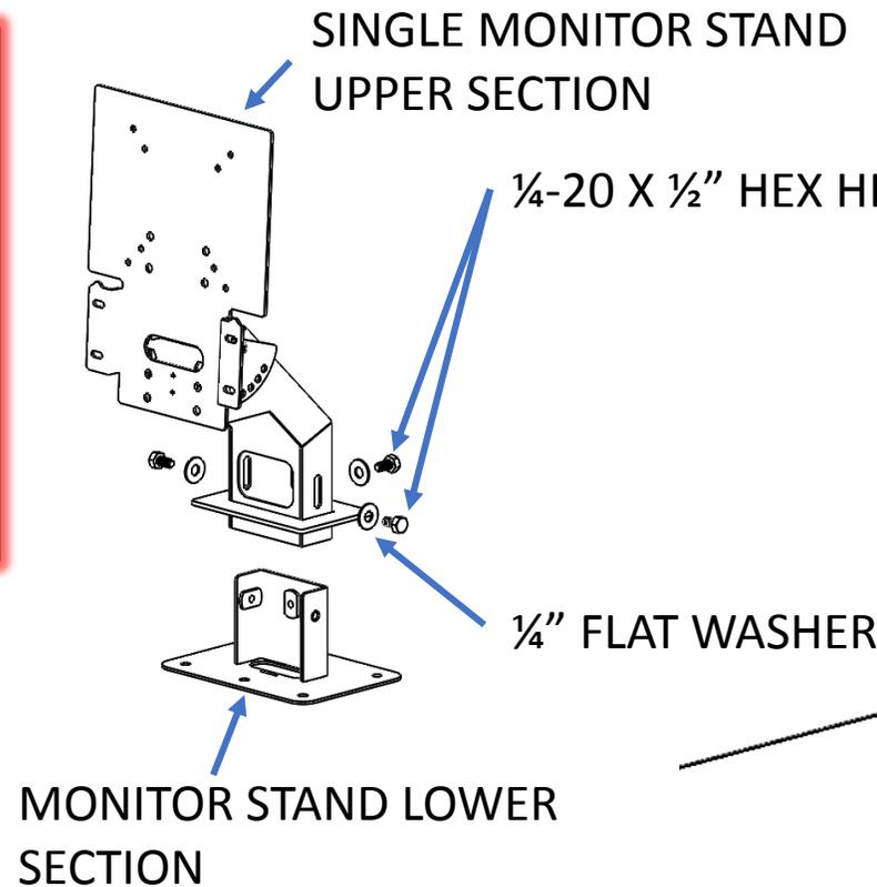
MONITOR STAND LOWER SECTION ALREADY INSTALLED TO UNDERSIDE OF COUNTERTOP
