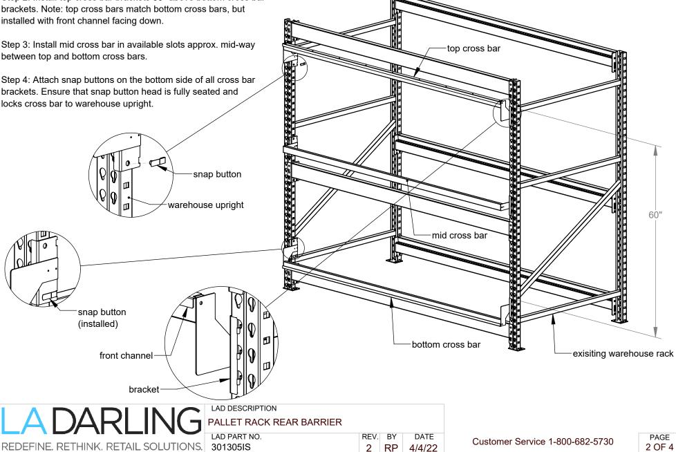
Step 5: Slide hardboard panels into channel on top and bottom cross bars. Note: 4' wide kits will only use one panel.
