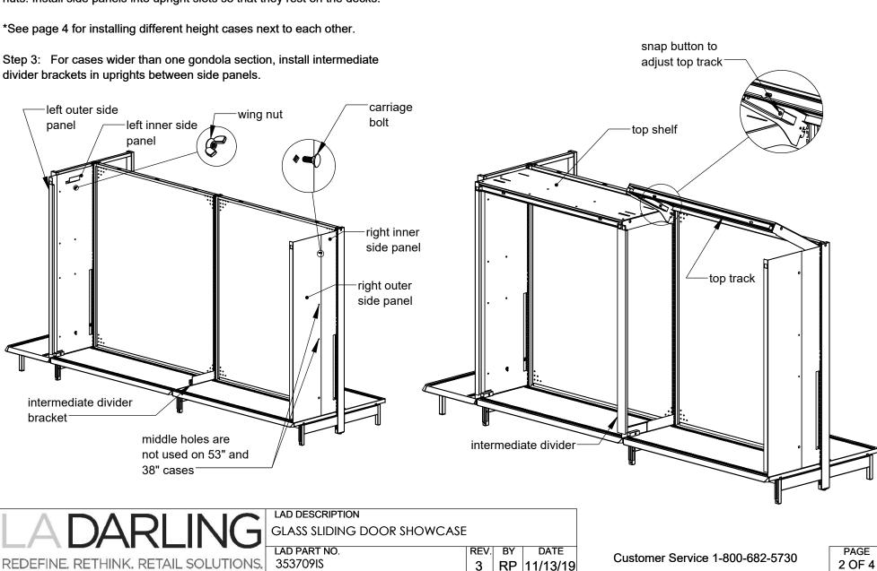
Step 4: Install top shelves level with the top of the side panels. Adjust
