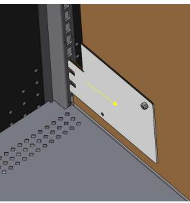
Step 3: Slide the bracket out until the top hole of the bracket line up with the hole in the side panel. Secure bracket with screw and nylon lock nut. The nylon nut should be inside the case. (LEFT)
