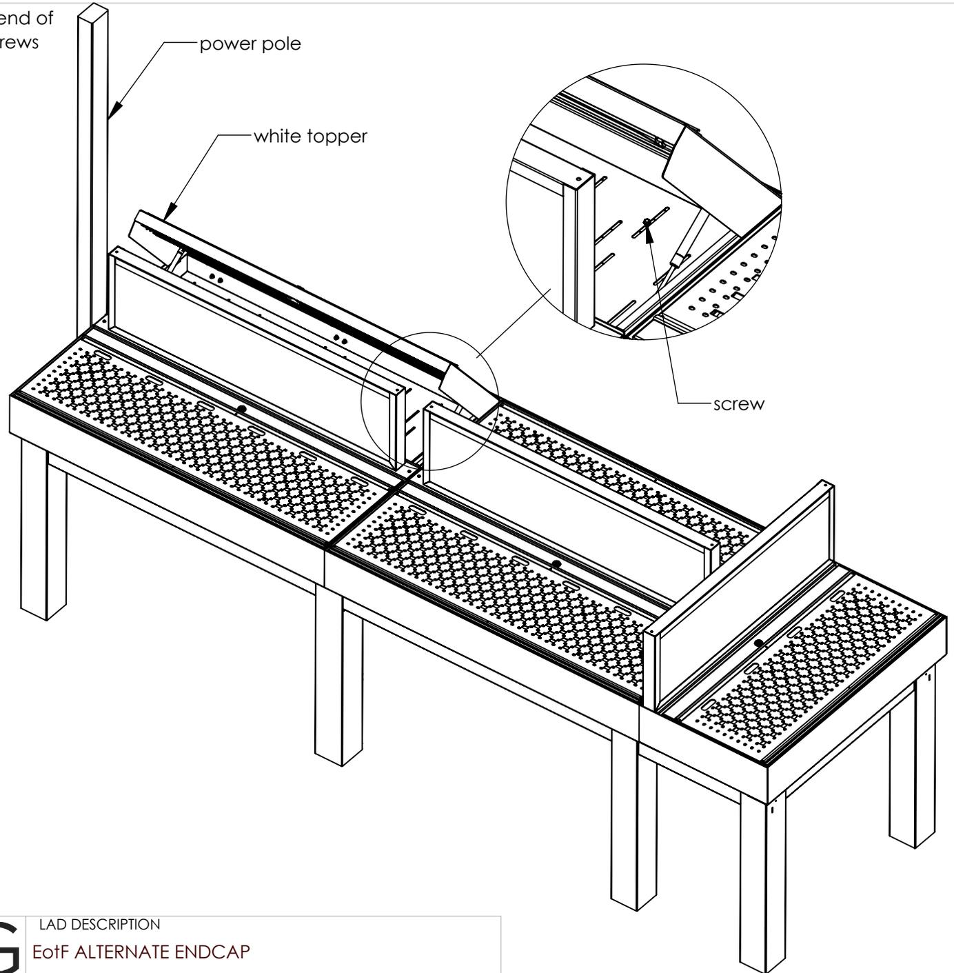
Step 2: Remove 2 TEKS screws from end of receiver box.
