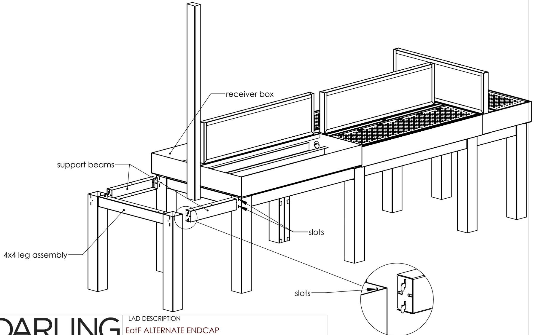
Step 4: Ensure support beam hooks are fully seated in slots, and secure them with a TEKS screw on each end.
