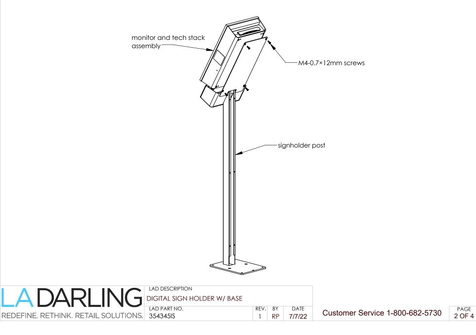
Step 3A: For sign holders positioned on top of vignette base, secure baseplate using four TEKS screws. Skip to step 5.
