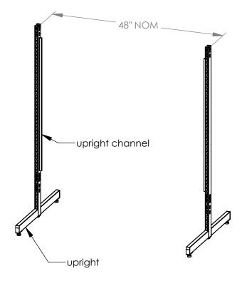
Step 2: Insert tabs of cross channel into slots at bottom of uprights. Seat in place by tapping on each end of cross channel.
