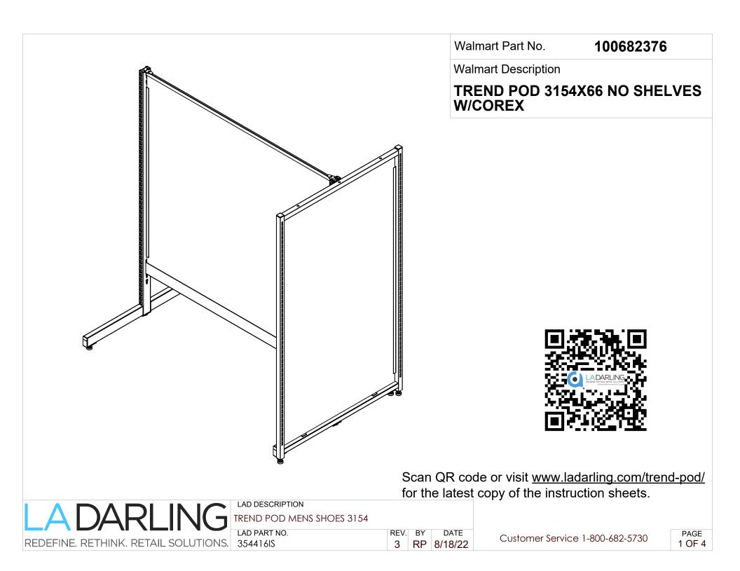
Step 1: Hold uprights about 48" apart with levelers resting on the floor and the channels facing each other. Step 2: Insert tabs of cross channel into slots at bottom of uprights. Seat in place by tapping on each end of cross channel.
