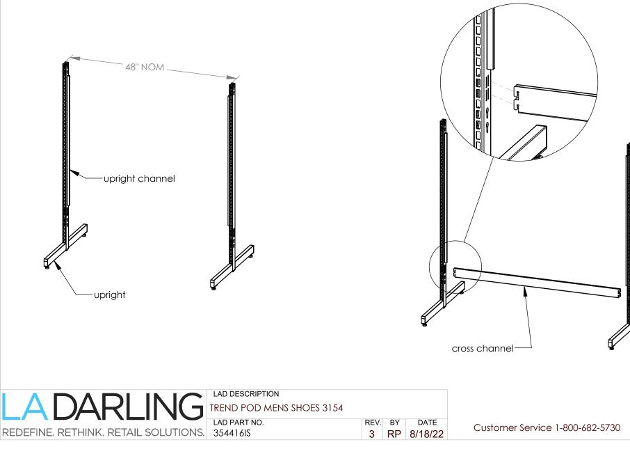
Step 3: Slide corrugated panel into channels on uprights and cross channel.
