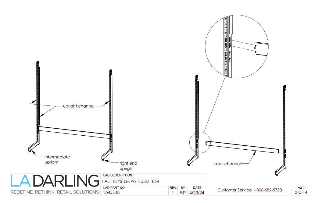
Step 3: Slide hardboard panel into channels on uprights and cross channel.
