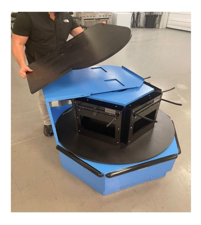
STEP 9 Remove the (2) machine screws that attach the Underside Panel to the top of the Carousel Tower.
