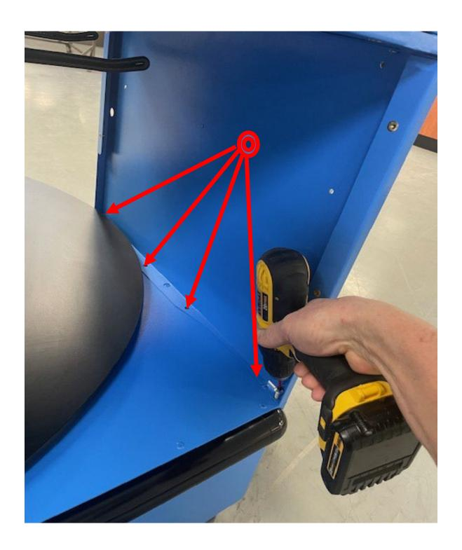
STEP 11 Remove the (4) machine screws from the other side and install later on other side (step 18).
