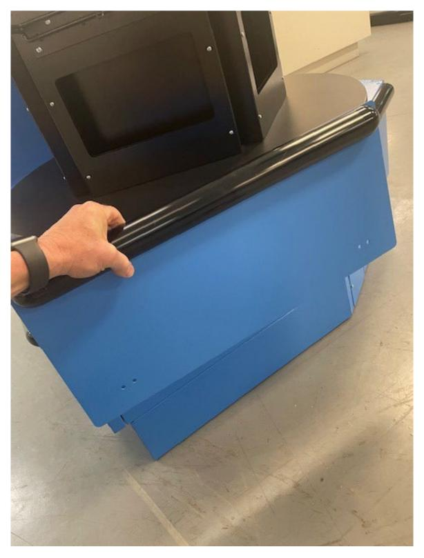
STEP 3 Relocate the Bumper Cover to opposite side, in alignment with the Upper side Panel
