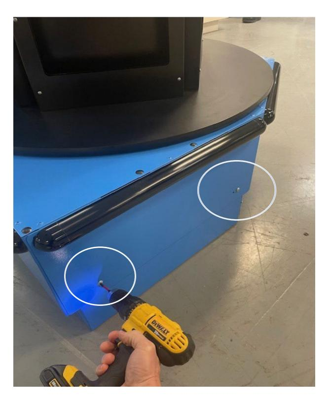
STEP 2 Remove Cover by pulling upward to disengage the two clips on the backside of the panel
