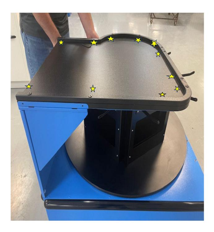
Placing one of the Allen wrenches on the top connector and one on the bottom connector, loosen \ remove each of the (11) bolts. Once removed – the HDPE top trim pieces will separate from the top HDPE deck.
