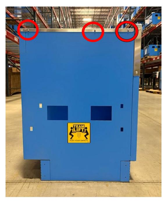
Remove access panels and adjust levelers (if needed) to level table top to scanner table. (Qty. (6) levelers).
