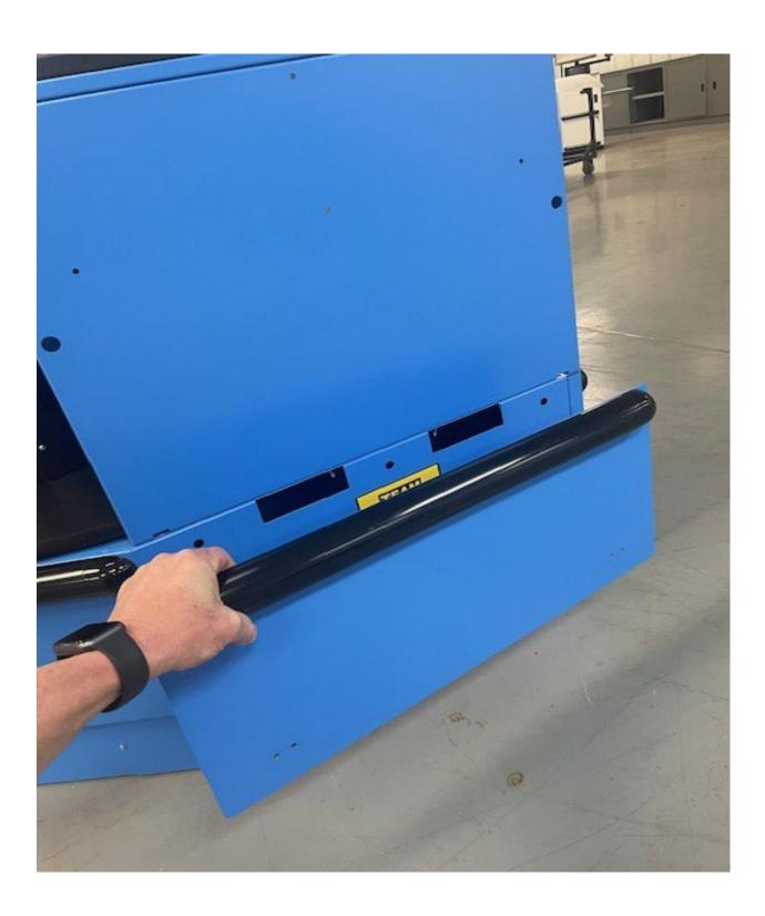
Rotate the Carousel unit, (180 degrees), to align the newly created attachment side of the Carousel unit with the existing Front Conveyor. Reattach the Bumper Cover to the opposite side of the carousel using the same machine screws that were previously removed.
