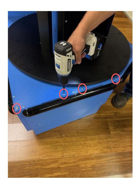
Remove the Frame Assembly from the Carousel Unit - as shown below – then re-attach it to the side where the Bumper Cover was relocated (Refer back to STEP 4)
