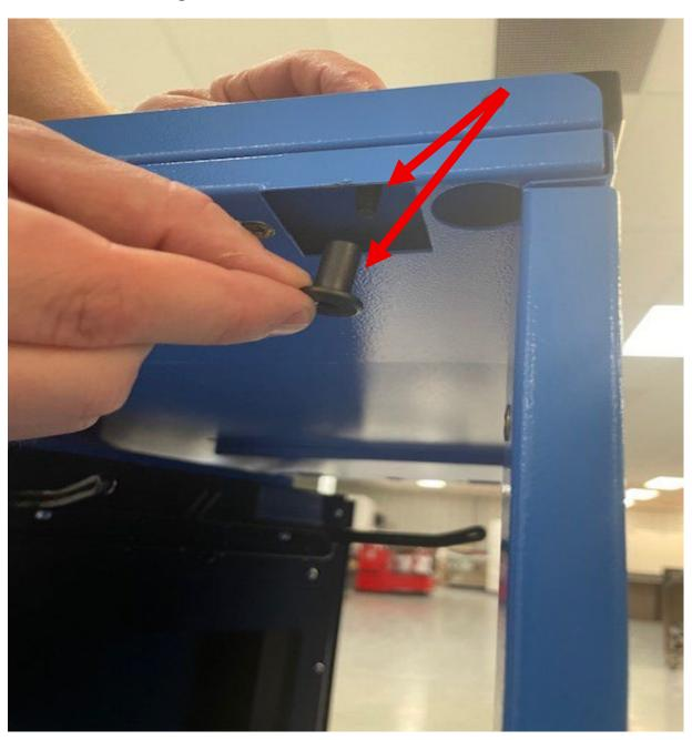
STEP 16 Re-install Corner Bracket to the End Panel and Underside Top Support Panel – using the original (5) machine screws previously removed.
