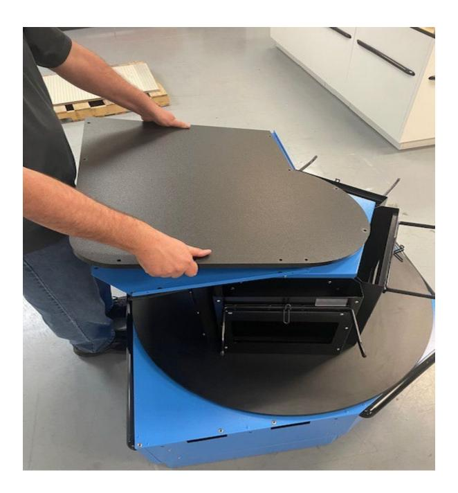
Once the Frame \ Top Assembly – from STEP 13 &14 – has been reinstalled on the opposite side - Reverse the assembly order of the above STEPS and reattach all components to complete the Conversion.
