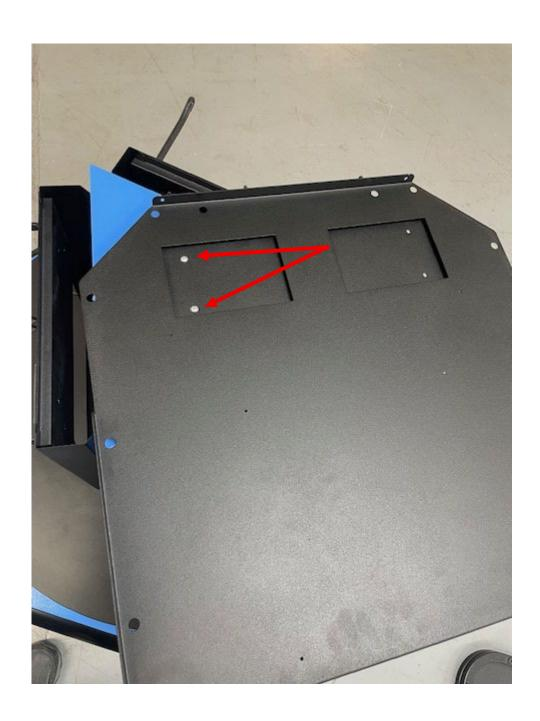
STEP 10 Remove the (4) machine screws that attach the End Panel to the Carousel.
