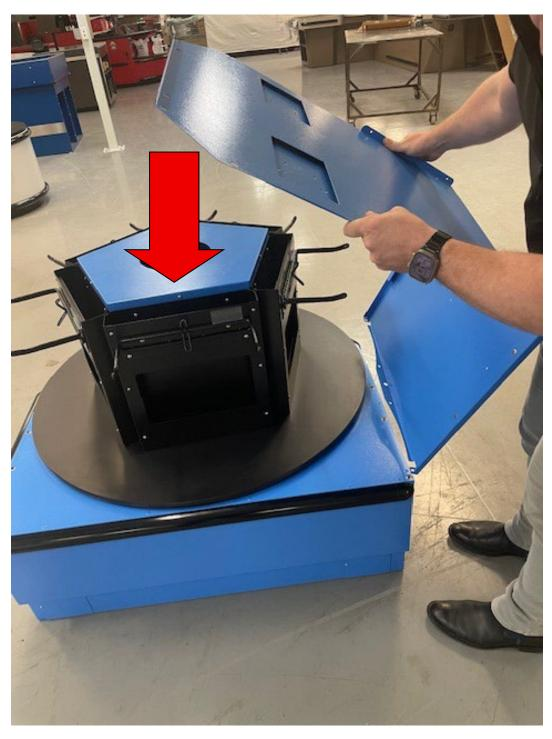
Flip the HDPE top over – to expose the opposite side - then place it on top of the Underside Support Panel to convert it to the opposite handed unit.
