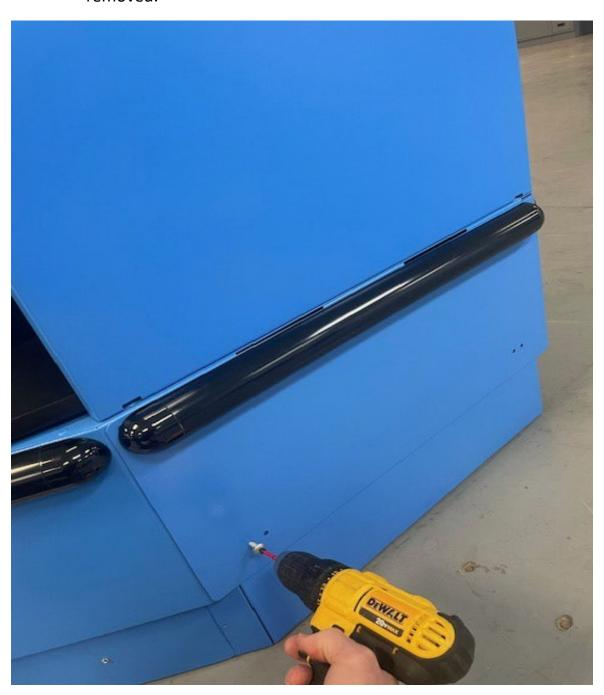
STEP 5 Remove the screws attaching the Corner Gusset and HDPE top to the Underside Panel
